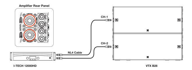
Alternatively, a cable splitting an NL4 to two NL2 connectors can be used, which allows connecting a pair of B28 subwoofers using a single four-conductor NL4 cable. This can reduce cabling requirements by a factor of two. The NL4 connector for channel A on the amplifier must be used in this configuration, as it carries both channel signals, while the channel B connector does not.
