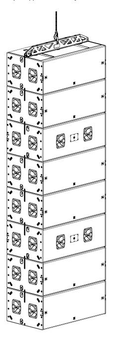
In some cases, asymmetric arrays are unavoidable, especially when the arrays are configured in blocks of four cabinets. In these cases, coverage tends to be biased towards a specific direction, but strategic placement can help shape coverage to the specific needs of a venue. Use LAC-3 to design such arrays.
