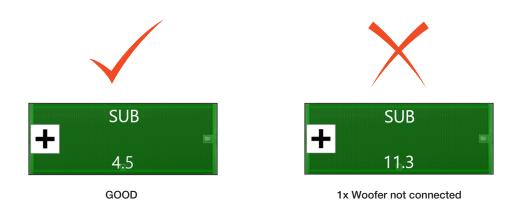
The measurements recorded by Performance Manager are susceptible to drift based on variables such as temperature, cable length, wire gauge, and usage conditions. Parameter variations such as temperature will be common across all B28 enclosures in use, so all B28 subwoofers in a system should measure similarly. An enclosure measuring significantly different than others (by as much as several ohms) indicates something wrong with that enclosure.
