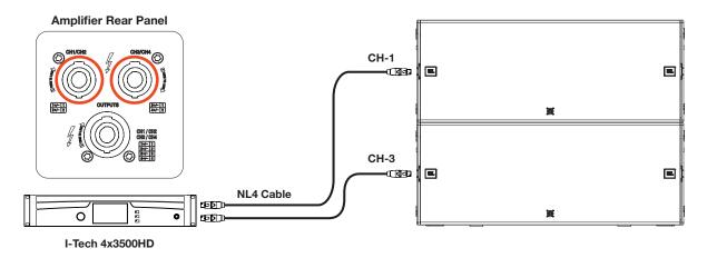
Alternatively, a cable breaking the NL4 connector out to two NL2 connectors can be used to drive one B28 each from amplifier channels 1 and 2. A four-conductor NL4 cable is employed in this arrangement, reducing cabling requirements. Amplifier channels 3 and 4 remain available for driving a full-range product, such as the VTX A8.
